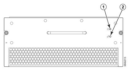
Figure 29. Blower assembly LEDs
